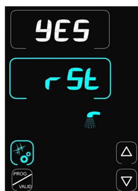
Reset water counter
