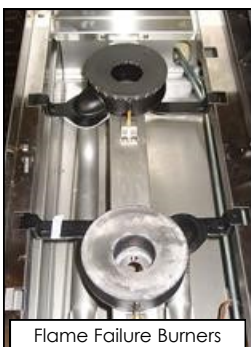
Flame Failure Burners
